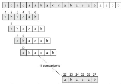
**Figure 23.2:** Example run of the brute-force pattern matching algorithm. The algorithm performs 27 character comparisons, indicated above with numerical labels.
