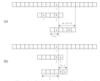
**Figure 23.4:** Illustration of the jump step in the BM algorithm, where l denotes last(T[i]). We distinguish two cases: (a)  $1 + l \le j$ , where we shift the pattern by j - l units; (b) j < 1 + l, where we shift the pattern by one unit.
