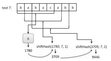
Figure 23.12: How a rolling-hash function works in the Karp-Rabin algorithm.
