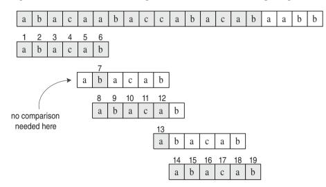
Figure 23.8: An illustration of the KMP pattern matching algorithm. The failure function f for this pattern is given in Example 23.2. The algorithm performs 19 character comparisons, which are indicated with numerical labels.
