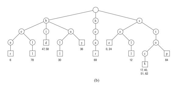
**Figure 23.15:** Word matching and prefix matching with a standard trie: (a) an example text that is to be searched; (b) a standard trie for the words in the text (with articles and prepositions, which are also known as *stop words*, excluded). We show external nodes augmented with indications of the corresponding word positions.
