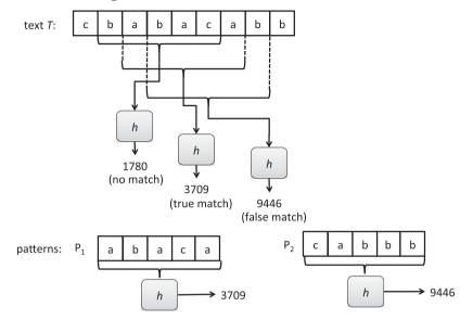
**Figure 23.10:** How the Karp-Rabin hash-based lexicon matching algorithm works. A hash value, h(X), is computed for each length-*m* substring, *X*, of the text. If it matches the hash value of a pattern, it is then confirmed as either a true match or a false match.
