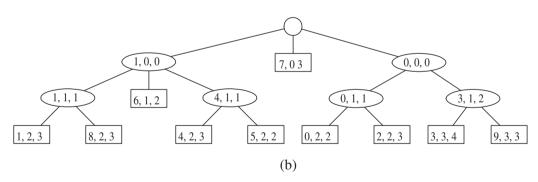
Figure 23.17: (a) Collection S of strings stored in an array. (b) Compact representation of the compressed trie for S.
